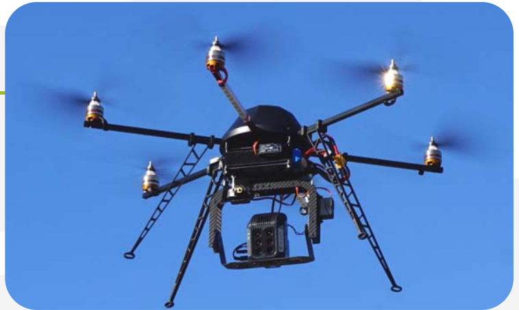
AIRPHEN embedded on UAV
