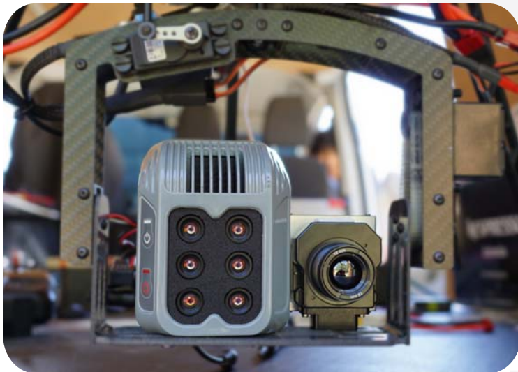
AIRPHEN + Thermal Camera FLIR Tau2
