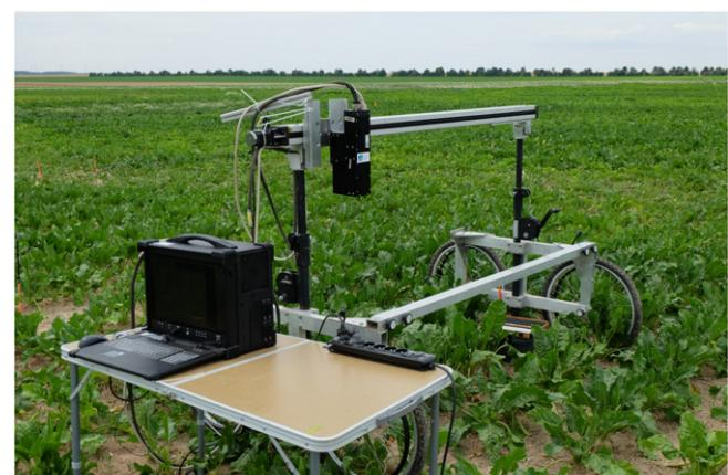
**Fig. 2.** Ground-based platform used for hyperspectral measurements.
